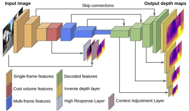
Figure 5. **Decoding architecture** used in our experiments. A single-frame depth network is augmented to include multi-frame cross-attention features (Section 3.2), generating depth maps at multiple scales in addition to those generated directly from multi-frame attention (Sections 3.3.1 and 3.3.2).
