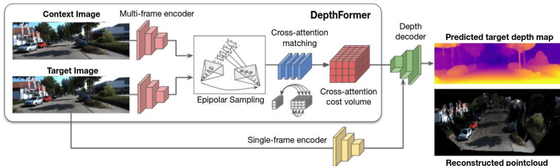
Figure 1. **Our DepthFormer architecture** achieves state-of-the-art multi-frame self-supervised monocular depth estimation by **improving feature matching** across images during cost volume generation.
