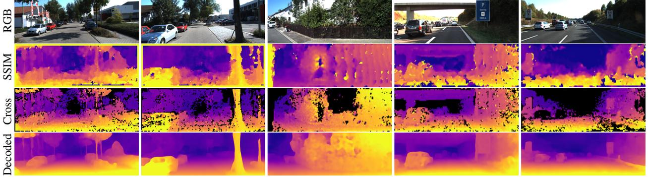
Figure 6. **Predicted depth maps** on the KITTI dataset, obtained from SSIM (argmin) and cross-attention (high response) cost volumes, as well as the decoded depth estimation output (full resolution). Corresponding quantitative results are reported in Table 2.
