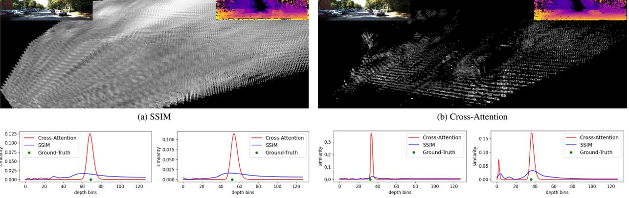
(c) Matching probability distribution along depth bins for different pixels relative to their depth-discretized epipolar candidates. The blue line shows SSIM values (Equation 9), the red line shows cross-attention values  $\alpha_L$  after refinement (Section 3.2), and the green dot marks the corresponding ground-truth depth value (used only for comparison).
